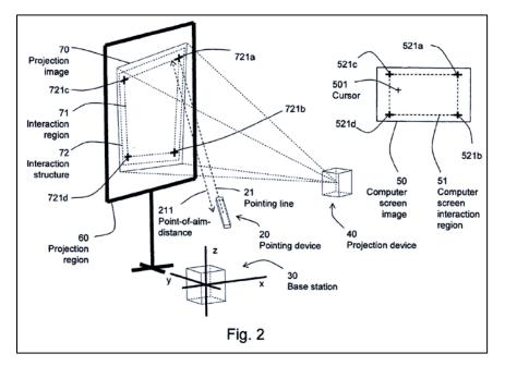
Id. fig. 2. The pointing device (20) can measure its location and orientation relative to the projected image (70), and use that measurement to determine where on the image to display the cursor. Id. col. 7 ll. 11–17. Claim 1 is exemplary and reads as follows:
